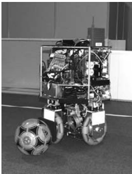
Fig. 2. Omni-directional mobile robot “Zen”
